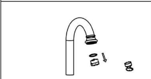
Type 2: Hidden Aerator with Aerator Key
